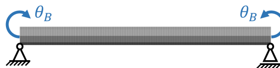
Figure 7. Boundary conditions for pure bending of a homogeneous beam.
